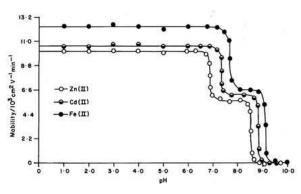
*Figure 1*: Mobility curves for the metal(II) – homoserine systems. Background electrolytes: 0.1 M perchloric acid and 0.01 M homoserine. The paper strips were spotted with 0.1  $\mu$ L of sample solution and glucose (for making osmotic correction).
