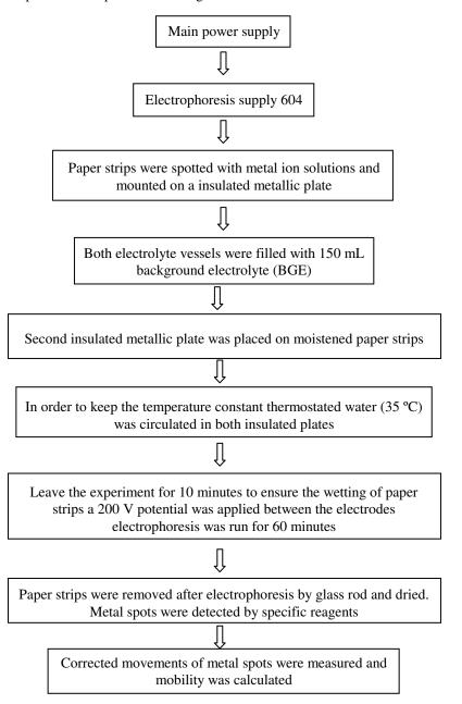
Figure 2: The scheme for paper electrophoresis set
